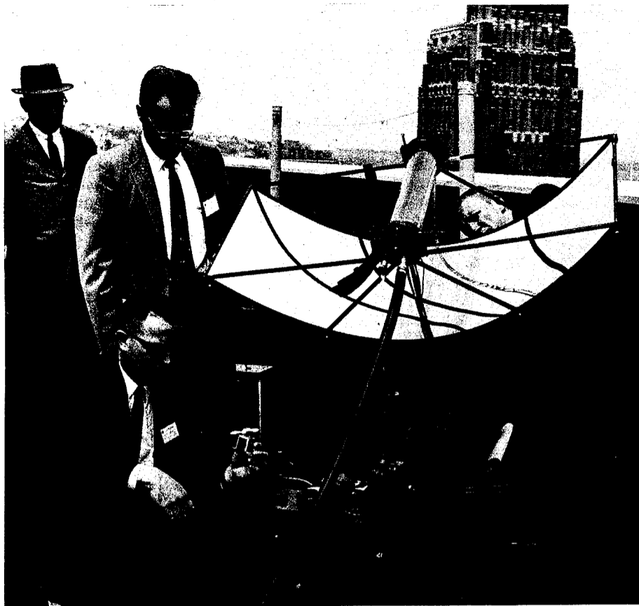
The thermoelectric generator pictured above demonstrated that it can convert solar energy of 2.5 watts, enough to operate a radio transmitter in space. Thus a possible competitor to the solar cell enters the space power source field.
